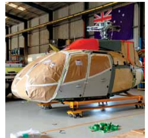
An EC130T2 arrives at Pacific Crown Helicopters from France as a "green" machine ready for assembly, painting and fit out to customer's needs and later delivery by Australian Aerospace to their client.
