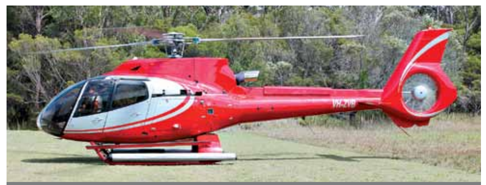
Almost finished. Final engine runs and checks. Fenestron is 50% quieter than an equivalent tailrotor, a good choice against the anti-noise lobby?
